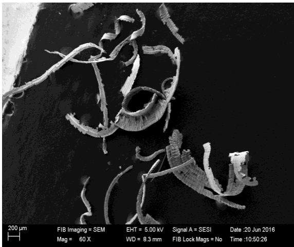
Fig 4.4 Thin continuous type chip formation
